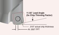
High-feed milling creates significant chip thinning due to an extreme lead angle. Feed rates must compensate for this to maximize productivity. The figure at left shows an example of this condition. Adjusting feed rates to account for chip thinning creates cutting conditions that provide very high feeds (IPM), but at lighter depths of cut (DOC). See the specific instructions for each size of high-feed insert below to get the most of your Dapra RHINO-FEED<sup>™</sup> product!
